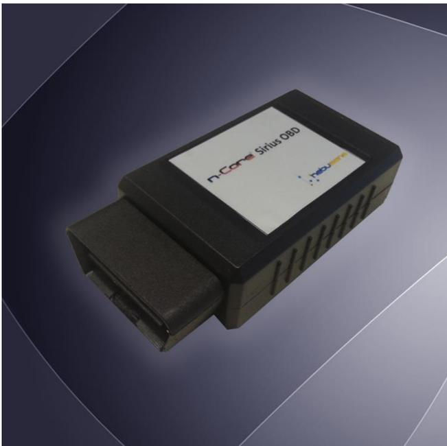
The new *Sirius OBD* device is part of the **n-Core platform**, developed by Nebusens. The n-Core platform offers a complete set of hardware and software tools that can fit all your necessities when developing and deploying wireless networks based on the IEEE 802.15.4/ZigBee international standard.
